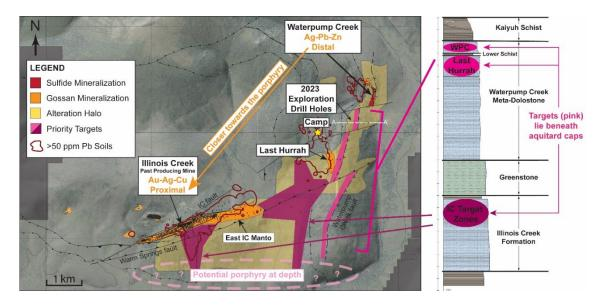
Figure 1. Plan map and stratigraphic column of the greater Illinois Creek region: including the past-producing the Illinois Creek Mine, and Waterpump Creek and Last Hurrah prospects. See our website for the A to A' Last Hurrah drill section.
