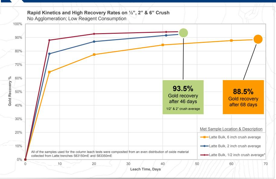
\* ½ inch column performed at a temperature of 4° C to simulate cold climate leaching. 2 inch and 6 inch columns performed at ambient lab temperature (22° C) due to lab refrigerator not being able to accommodate column size.
