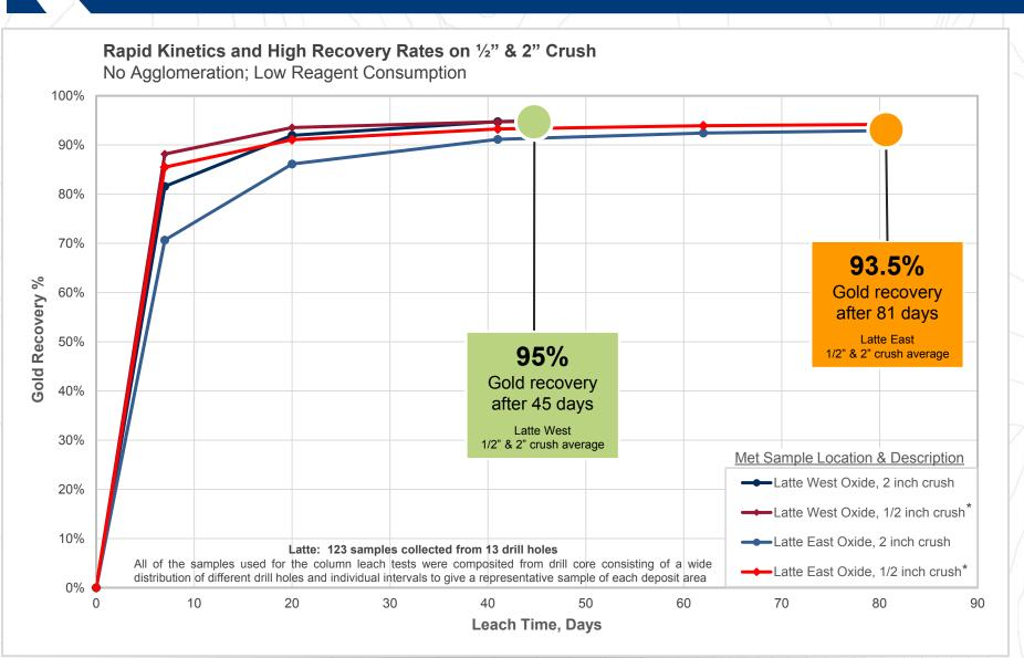
\*  $\frac{1}{2}$  inch columns performed at a temperature of  $4^{\circ}$  C to simulate cold climate leaching. 2 inch column performed at ambient lab temperature (22° C) due to lab refrigerator not being able to accommodate column size.
