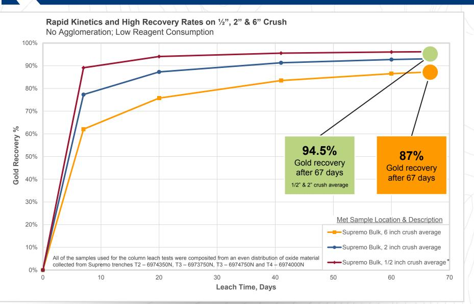
\*  $\frac{1}{2}$  inch column performed at a temperature of  $4^{\circ}$  C to simulate cold climate leaching. 2 inch and 6 inch columns performed at ambient lab temperature (22° C) due to lab refrigerator not being able to accommodate column size.
