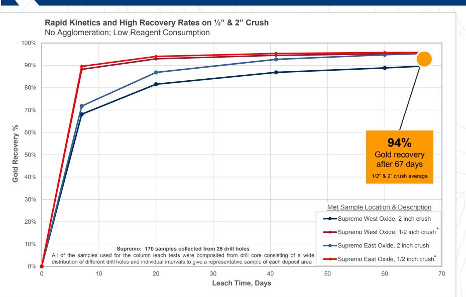
\* ½ inch columns performed at a temperature of 4° C to simulate cold climate leaching. 2 inch and 6 inch columns performed at ambient lab temperature (22° C) due to lab refrigerator not being able to accommodate column size.
